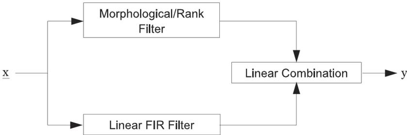
Fig. 5. Structure of the MRL filter.
